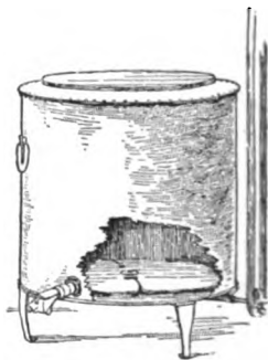
FIG. 81.—Pasteurizer with mechanical agitator.
